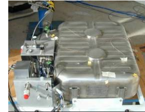
conformable LH 2 tank (8 kg)
