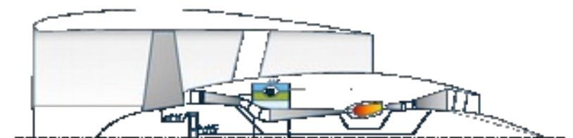
Type D Electric machine encircling core engine, motor connected to PT shaft via coupler
