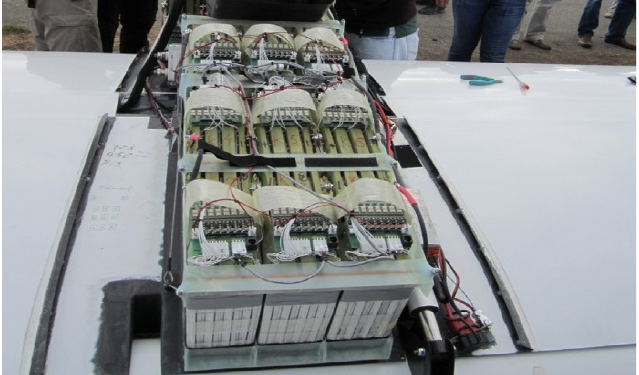
Specific challenge: half-ton Li-Po battery
