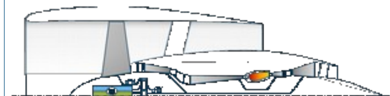
Type C Electric machine integrated with fan hub, motor connected to PT shaft
